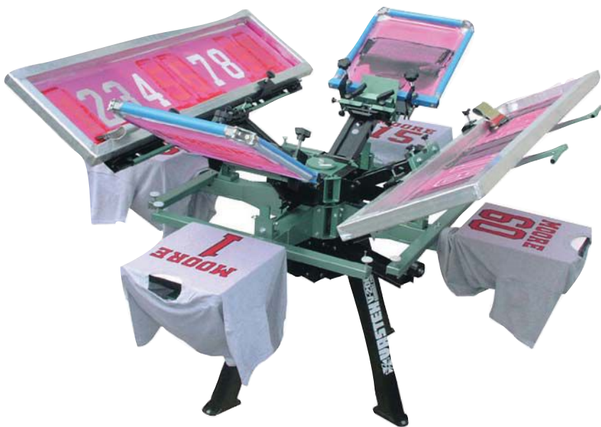
The Vastex DiGiT Numbering System is a press attachment that can produce up to 120 shirts per hour. Available from Atlas Screen Supply Company (circle 128 on Free Info Card).
