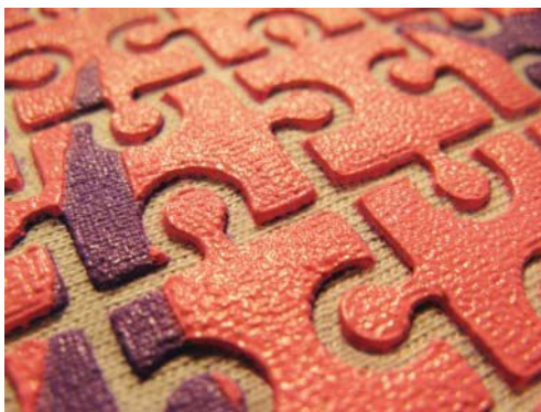
▲ High-density inks create sharp, defined prints in three dimensions.
