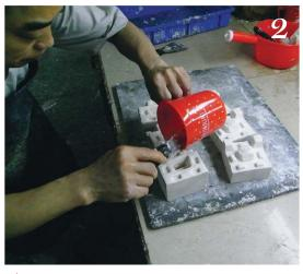
↑ Pouring the liquid poly-resin material into the silicone mold.
