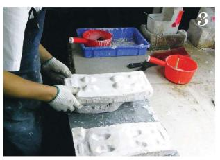
↑ Carefully removing the raw casting from the mold.
